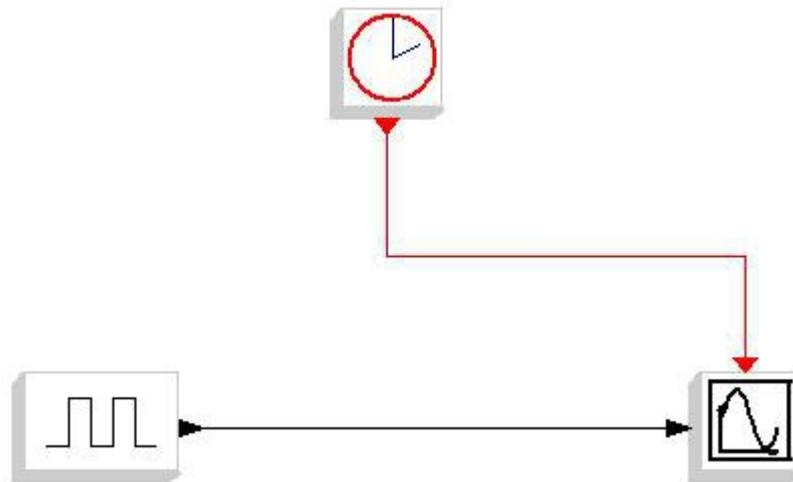
Fig. 1.7: Diagram comprising the synchronization block CLOCK c.
