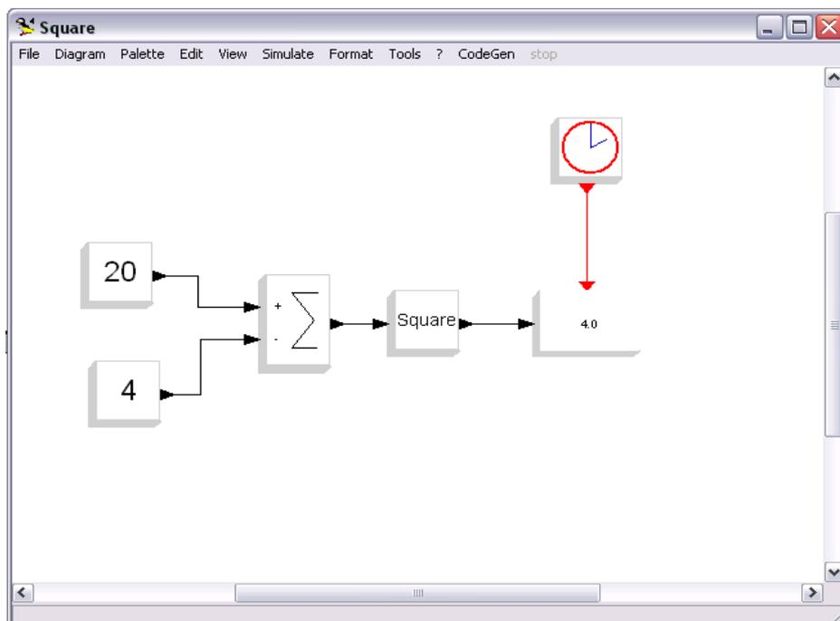
Fig. 1.30: Scicos scheme containing the new block created.
