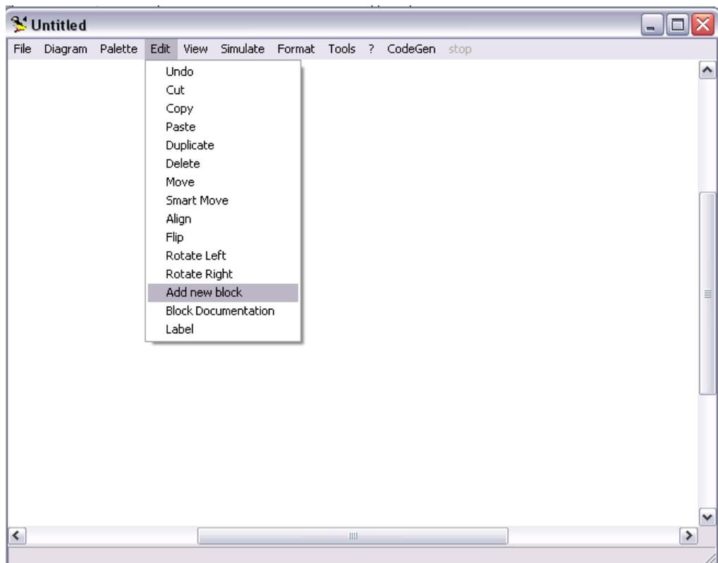
Fig. 1.27: Path to add a new block to Scicos.
