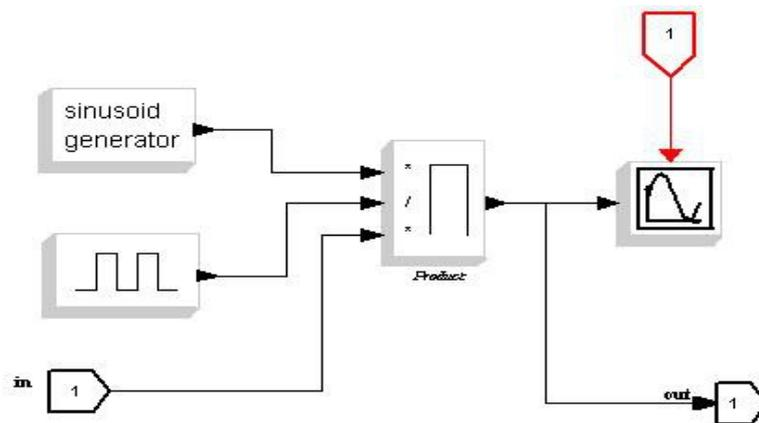
Fig. 1.21: Inner view of the Superblock created with the addition of input and output label.
