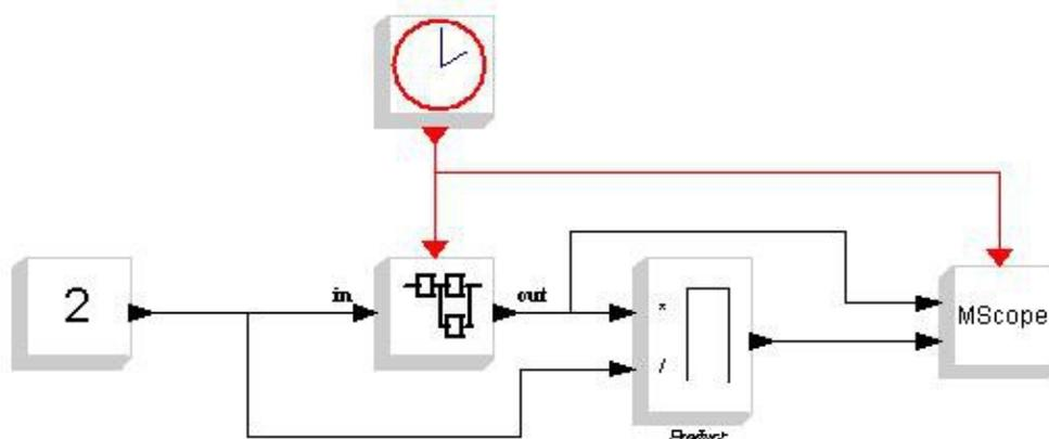
Fig. 1.22: Diagram of Fig. 1:20 after addition of labels of input and output from the superblock .
