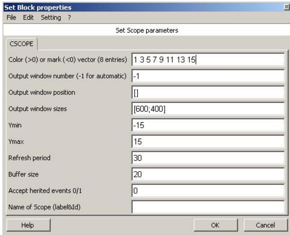
Fig. 1.6: Setting window of block CSCOPE.
