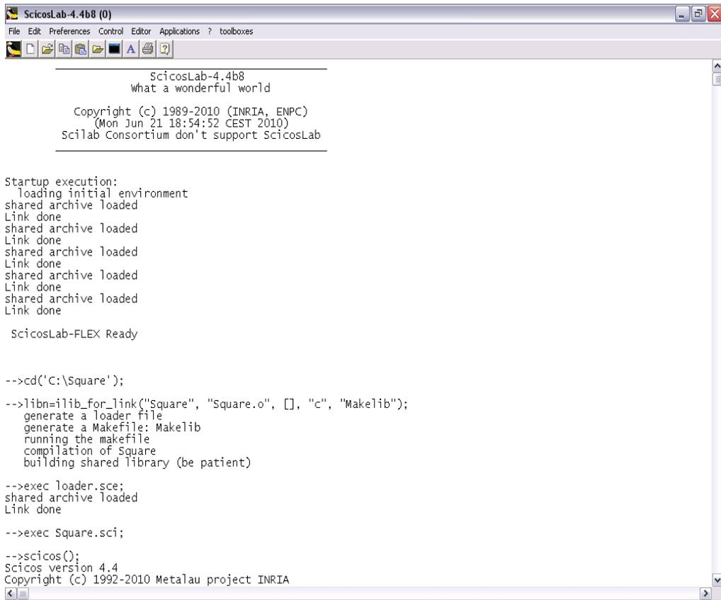
Fig. 1.26: Compilation and linkage of computational and interfacing function in ScicosLab / Scicos.
