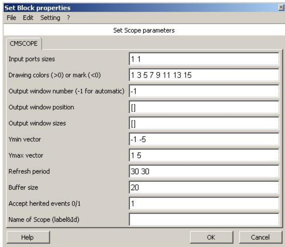
Fig. 1.19: Setting window of the block C SCOPE (Default settings)
